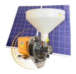
The Agsol Hammer Mill is a 48V DC grain milling machine that can be offered in electric format with an AC-DC power supply, or in solar format with charge controller, battery pack, and solar panels.
